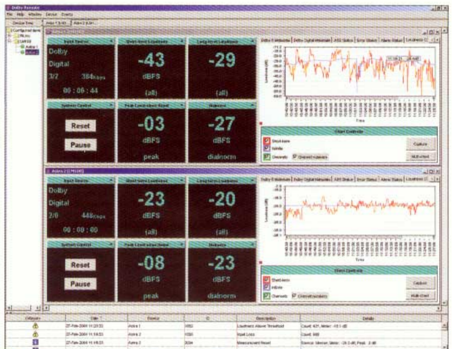
With the new remote software application for the LM100, variations in loudness can be logged simply and reliably
